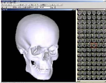
3D solid and surface models can be created from any types of volumetric images for modeling and rapid prototyping applications.
